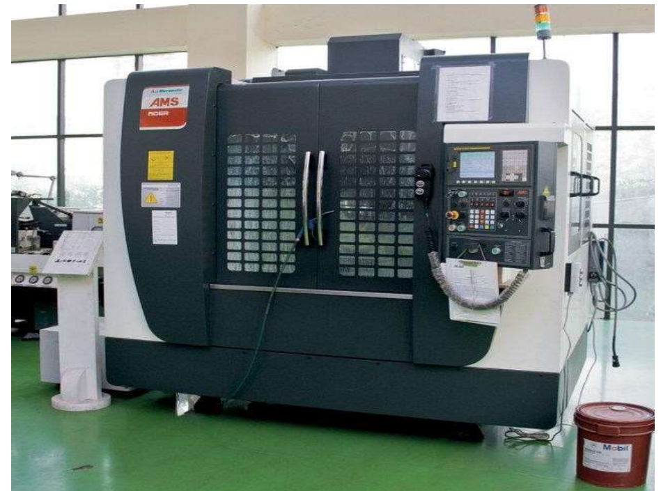
Newly added VMC Machine with Rotary Table which enhance quality & accuracy of component in minimum cycle time. Pallet Changer VMC added.
