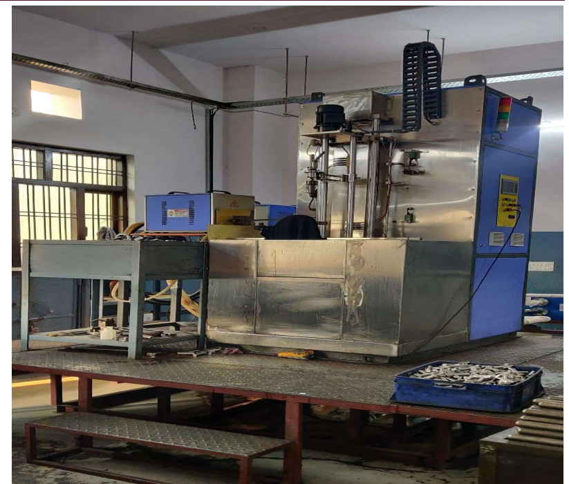
Newly added Induction Hardening Machine with Tempering Furnace.
